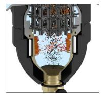
subsequent expulsion of sludge while the system is still running. Since the magnetic ring is positioned outside the separator body, the hydraulic characteristics of the device are not altered.
